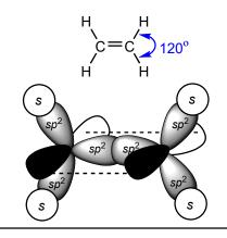
**Trigonal planar** orientation of sigma bonds in ethylene ( $sp^2$  hybridization). A pi bond is formed by overlapping p orbitals that are orthogonal
