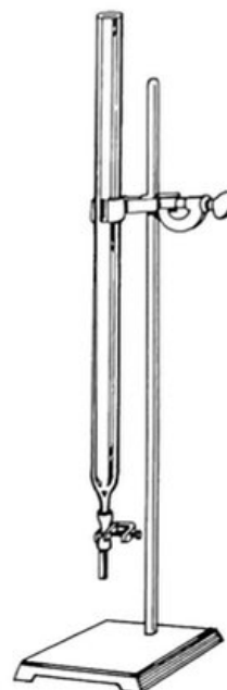
FIG. 9.3 A chromatographic tube on a ring stand.
