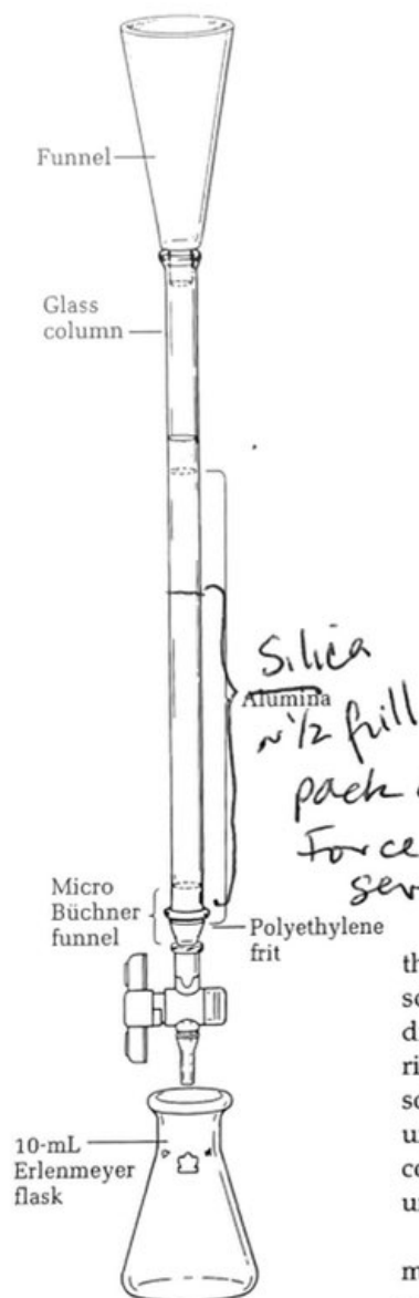
FIG. 9.1 A microscale chromatographic column.
