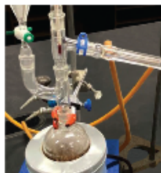
In a steam distillation, the essential oil of a plant is isolated as it co-distills with water.
